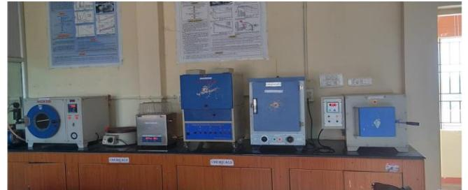
Hot Air Oven, Furnace, Incubator
